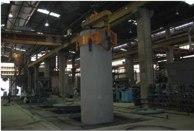
Gấp ống - Remove the core of the cast area
