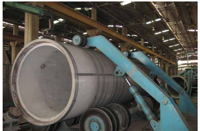
Quấn thép - Steel winding
